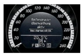
Tyre pressure loss warning system
