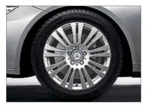
17-inch multi-spoke light-alloy wheel (standard for 4 and 6-cylinder)
