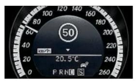
Speed Limit Assist even warns you about temporary speed limits
