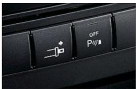
Button on centre console for belt feeder
