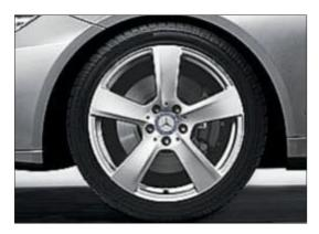
18-inch 5-spoke light-alloy wheel with mixed-size tyres (optional, Code R32, standard for 8-cylinder)
