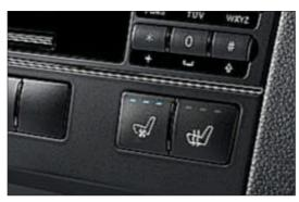
Climatised seats with button for seat ventilation/seat heating
