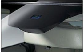
Rain sensor and light sensor for Headlamp Assist
