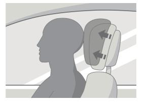
NECK-PRO head restraints The NECK-PRO head restraints are sensor-controlled. After deployment, they can be returned to their original position by hand
