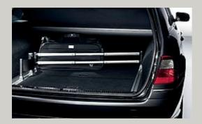
EASY-PACK load-securing kit To make sure that everything stays where you want it to stay, both the Saloon and the Estate can be supplied with an EASY-PACK load-securing kit, which holds your cargo securely and tidily in place. It includes a telescopic bar which attaches to cargo rails at the sides and allows the load compartment to be divided flexibly into different zones. Round objects can be secured to the sides using the retractable load-restraining belt
