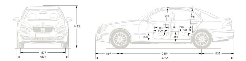
All measurements in millimetres. The dimensions shown are mean values and apply to standard-specification, unladen vehicles.
