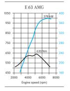
Torque (Nm) Output (kW)
