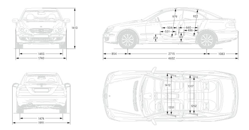
The dimensions shown are mean values (in mm) and apply to standard-specification vehicles carrying two occupants weighing 68 kg each
