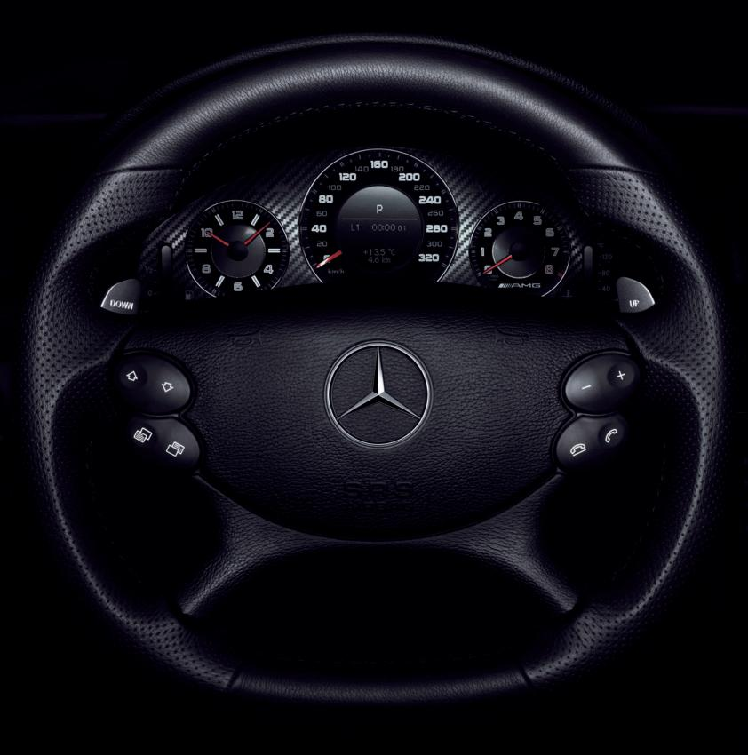
Experience that team driver feel: the AMG performance steering wheel, which measures 365 mm in diameter, is levelled off at the lower edge. The aluminium shift paddles make for fast and extremely ergonomic gear changes. And to help you keep track of what the CLK 63 AMG *Black Series* is capable of, the instruments in the carbon fibre dashboard feature red needles. Sit back and savour the exceptional sensory experience.
